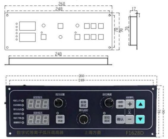
Figure 1. 4 F1628 Series Panel Installation Dimensions
