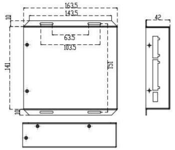
Figure 1. 2 F1627 Series Host Installation Dimensions
