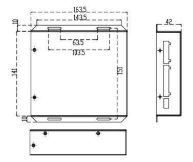
Figure 1. 5 F1628 Series Host Installation Dimensions Installation dimension drawing of pressure divider
