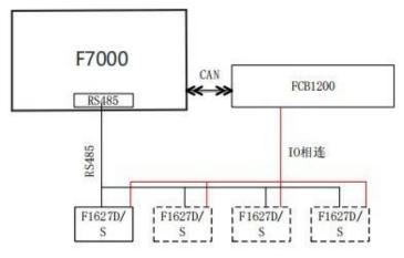
Note: All can only be the same type of F1627D or F1627S Figure 3. 21 F1627D/S and Shanghai Fangling F7000 series wiring diagram
