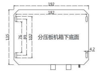
Figure 1.6 Installation dimension diagram of pressure divider
