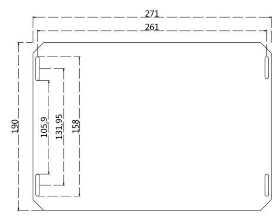
Figure 1.1F1620/F1621 installation dimensions of main engine
