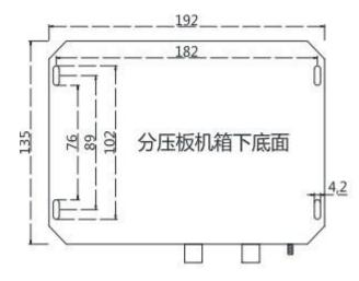
Figure 1.3 Installation dimension diagram of pressure divider
